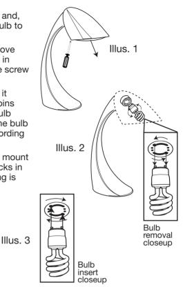
**CAUTION:** Before performing either bulb replacement or installation, be sure the lamp is unplugged, and if necessary, allow the bulb to cool.
